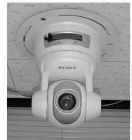
Fig.9 Pan-tilt camera
