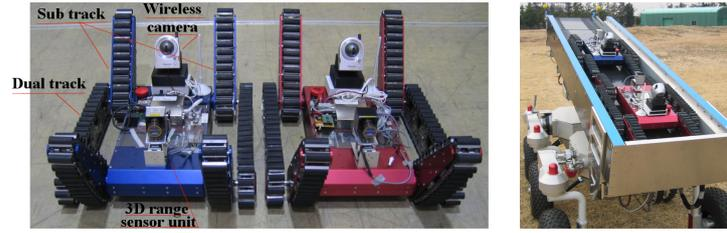
**Fig. 4.** The child robots “Muros-Piccolo” (left) and mounted on parent robot (right)
