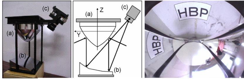
Fig. 8. Non-isotropic omnidirectional imaging system and obtained image
