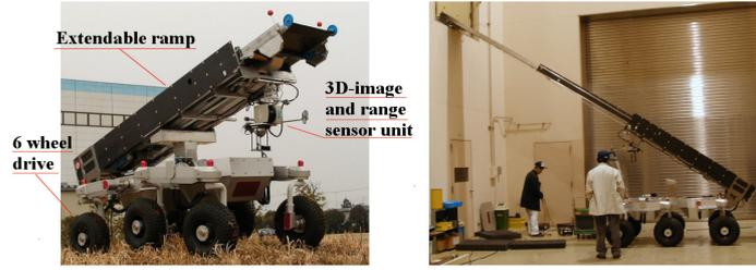
Fig. 2. An overview of the parent robot “Muros-Grande” and its ramp
