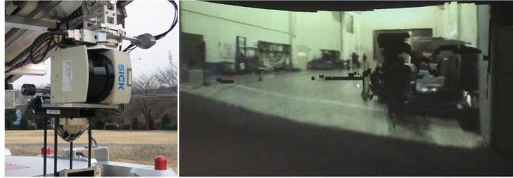
Fig. 9. Proposed sensor unit and obtained 3-dimensional information
