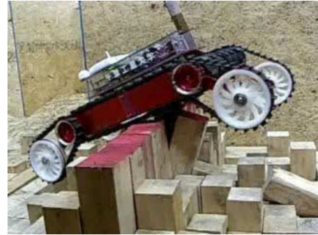
Fig. 1. Tracked vehicle with active flippers traversing on random step field
