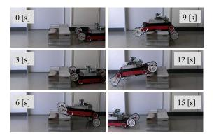
Fig. 9. Snapshots while traversing the step
