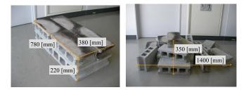
Fig. 6. A step comprising concrete Fig. 7. Complex terrain comprising blocks randomly positioned concrete blocks
