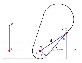
Fig. 3. Contact angle of the straight section of the flipper
