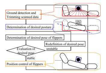
Fig. 2. Algorithm for autonomous controller for flippers
