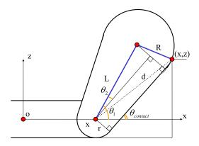
Fig. 4. Contact angle of the round section of the flipper
