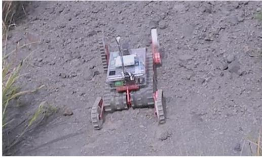
Fig. 7: Experiment on sandy slope (Kenaf)
