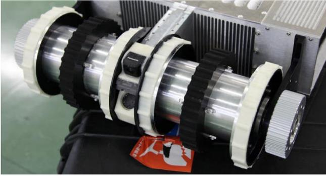
Fig. 10: Mechanism inside of tracks
