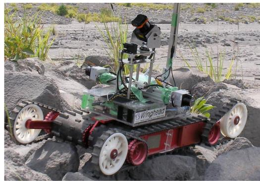
Fig. 4: Target robot platform Kenaf
