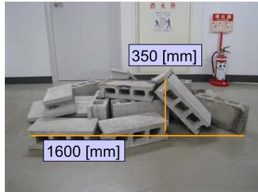
Fig. 5 A complex field comprising randomly positioned concrete blocks
