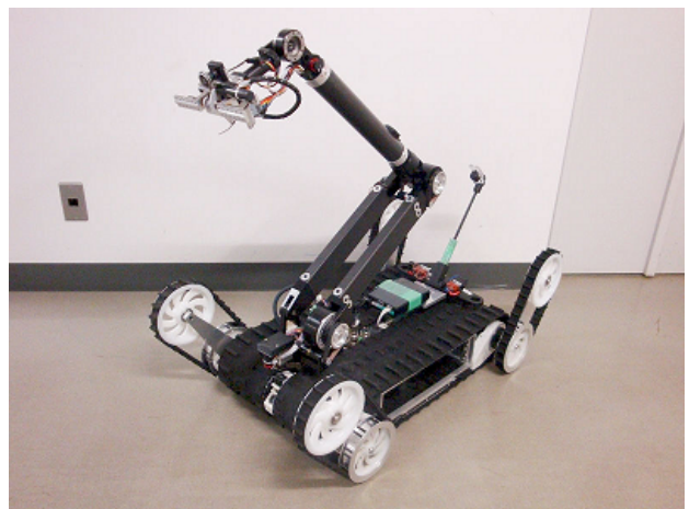
Fig.1 Rescue robot Quince with 6-DOF manipulator
