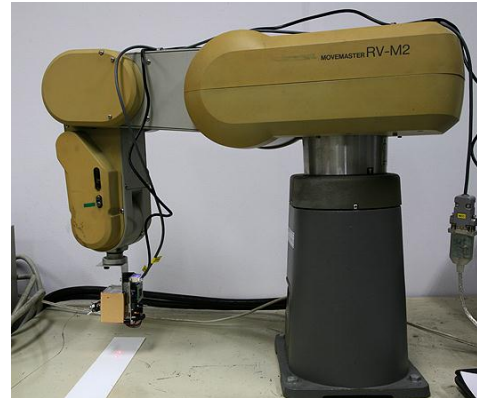
Fig. 3 Experiment environment. A robot arm moves the sensing device in a specified direction with accuracies of 0.1 mm in position and 0.1° in posture.
