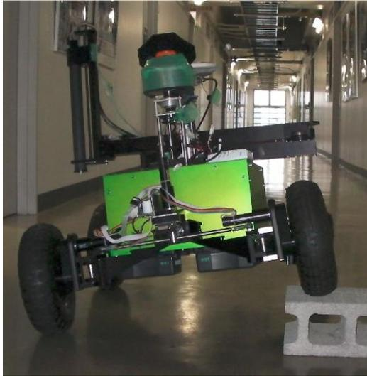
Fig. 2: Surmounting an obstacle using the rocker link
