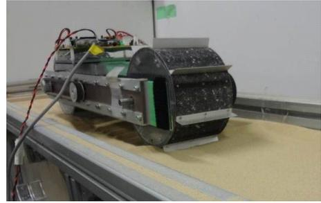
Fig. 8 Two-wheeled rover testbed (8 lugs)
