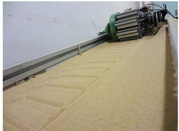
Fig. 10 Trajectory of testbed (verticality-penetration-lug wheel, slope angle is 12[deg])
