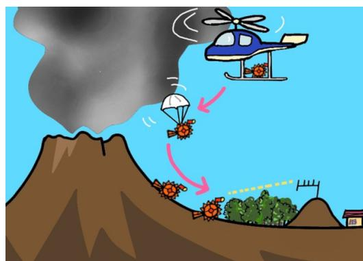
Fig. 1 Volcano exploration scenario using a multicopter and a mobile robot
