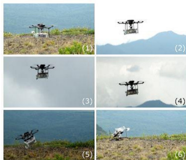
Fig. 4: Drop test of observation device
