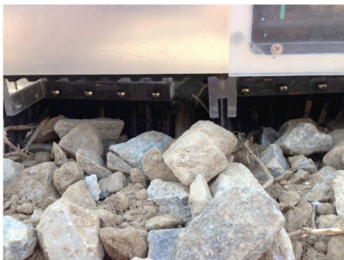
Fig. 12 Grousers on the slope
