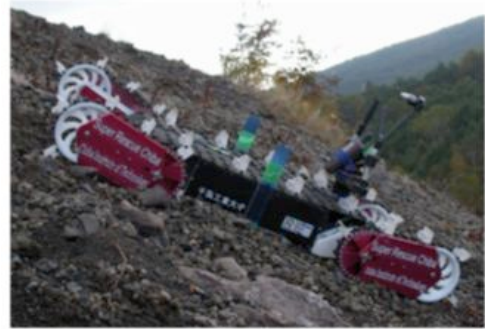
Fig. 1 Mobile robot in rough terrain "Quince"
