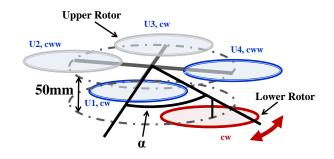
Figure 15. Details of the rotor arrangement in the experiment with two upper rotors and a lower rotor.
