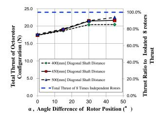
Figure 18. Total thrust of a octorotor UAV model at 6000 rpm based on experimental results.
