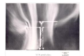
Figure 2. Visualized flow of coaxial rotor[1].
