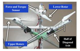
Figure 13. Measurement of thrust on two upper rotors and a lower rotor.
