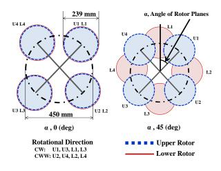
Figure 16. Top view of rotor arrangement for two angles at 450mm diagonal axis distance.
