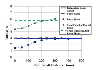
Figure 11. Thrust of overlapping rotors.
