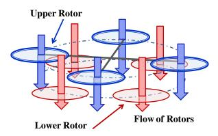
Figure 12. Concept of octorotor UAV avoiding wake interactions.
