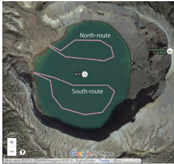
Fig. 5. USV path design on Google MyMaps. Designed paths are exported as a kml file. Note: a rope is stretched on an east-west centerline of Okama for conventional manned field-research. USV path must be designed to avoid the rope.
