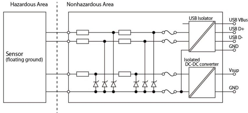
**Fig. 9** Isolated barrier circuit for USB devices.
