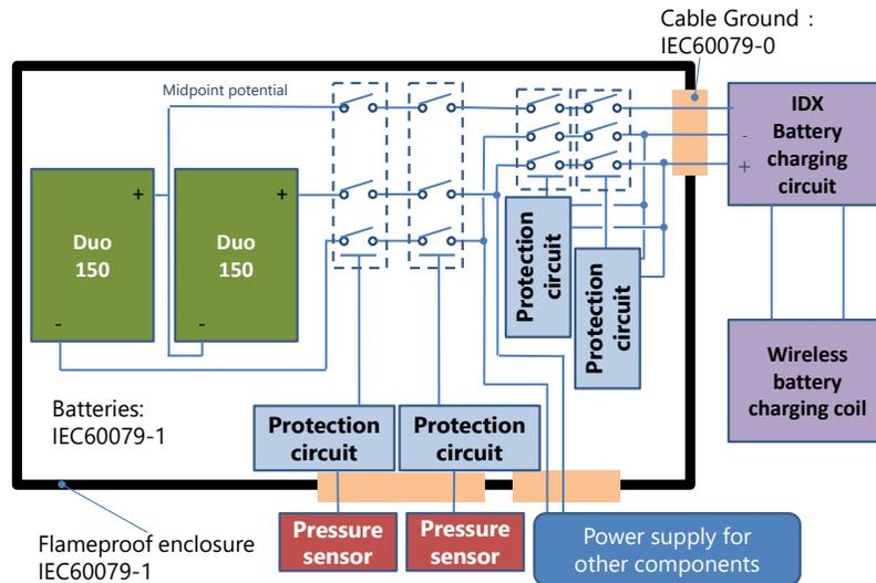
Fig. 4 Battery module diagram for AIR-K.
