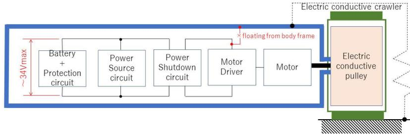
**Fig. 11** Earthing structure of AIR-K.
