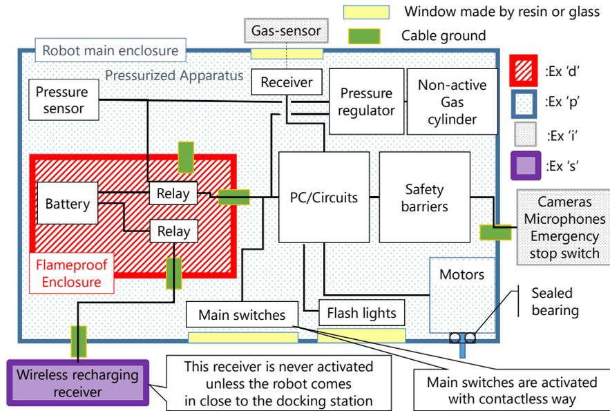
**Fig. 3** Block diagram of components of AIR-K.
