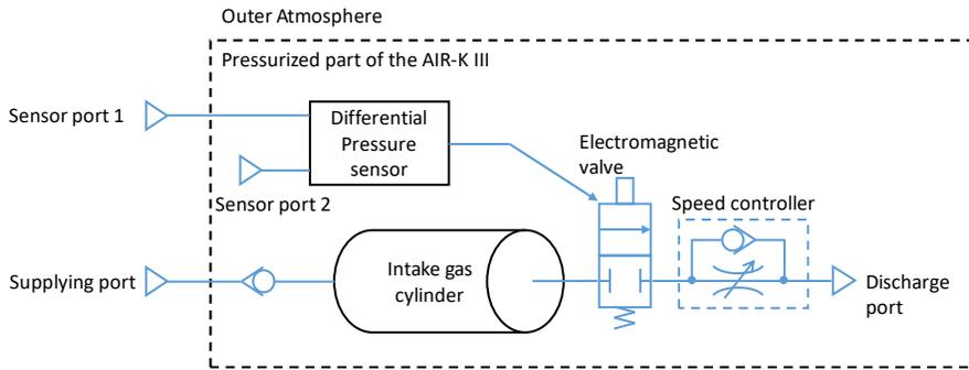
**Fig. 5** Diagram of pressurized apparatus for AIR-K
