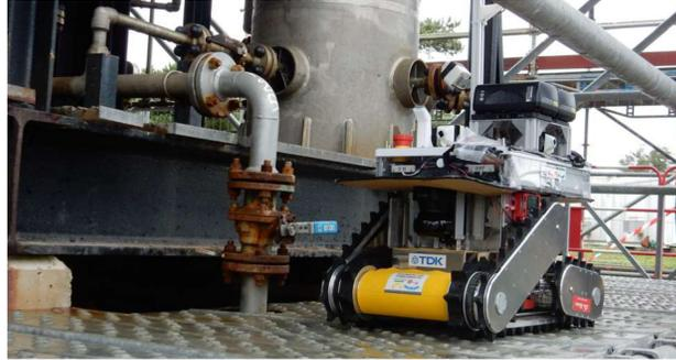
**Fig. 1** AIR-K prototype (non-explosion-proof version) in ARGOS Challenge.
