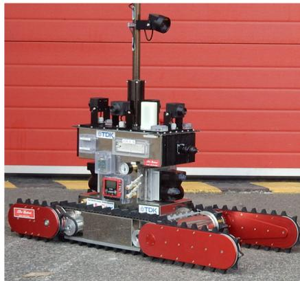
**Fig. 12** Explosion-proof robot AIR-K Ver.3.
