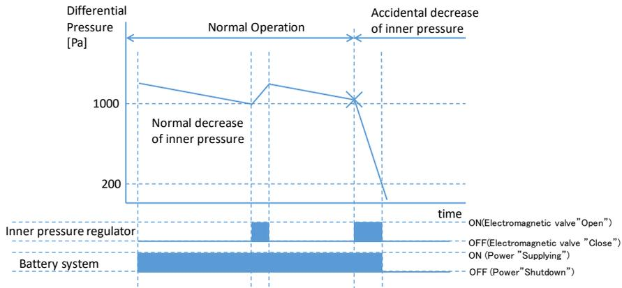
**Fig. 6** Relationship between pressure sensor and solenoid valve.
