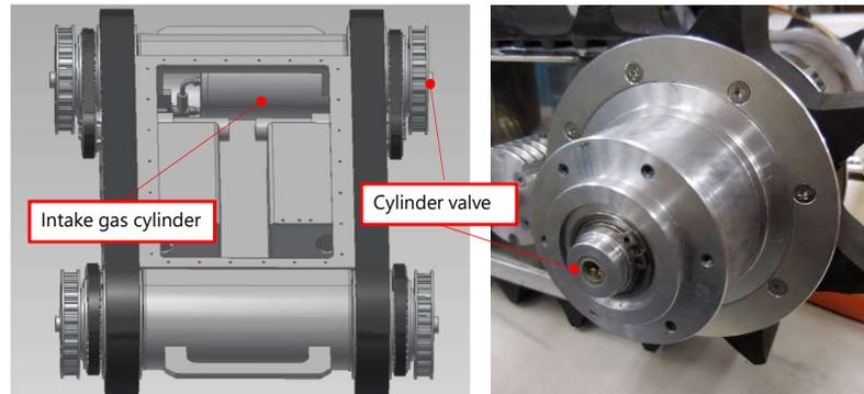
**Fig. 7** Intake gas cylinder and cylinder valve.
