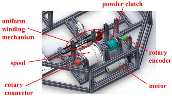
Fig. 4. Tether-tension-control winch and its control mechanism.
