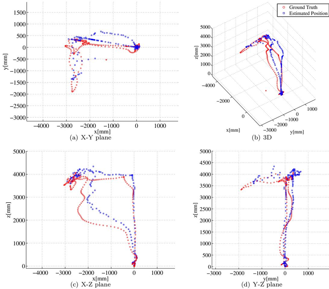
Fig. 8. Three-dimensional plot of measured/estimated MUAV's position.
