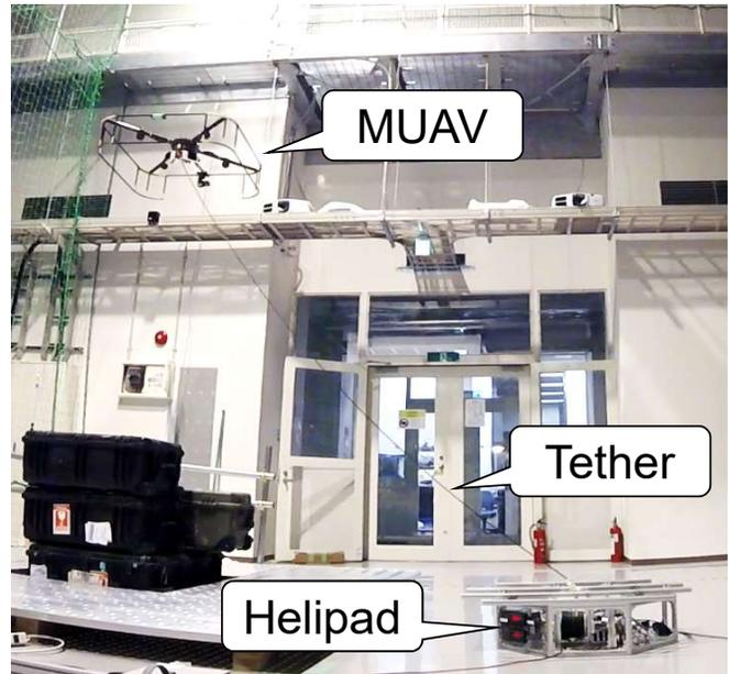
Fig. 9. Scene of flight experiment of tethered MUAV.
