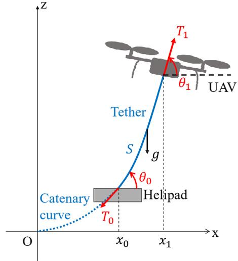
Fig. 2. Catenary curve of tether between MUAV and helipad.
