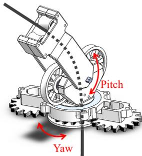
Fig. 5. Measurement Device of tether outlet direction.
