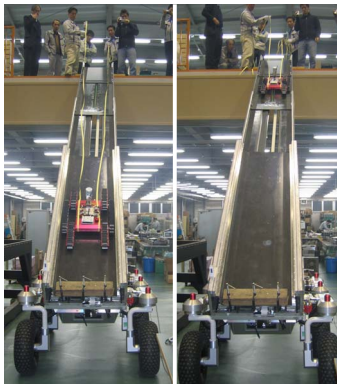
Fig. 10. Crawler climbing the rover's ramp up to the mezzanine
