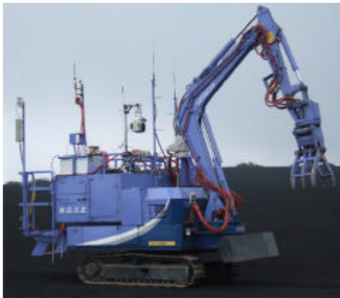
Fig. 1 Mobile Observatory for Volcanic Eruption (MOVE)
