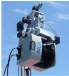
Fig. 2 Hung-type 3D range sensor
