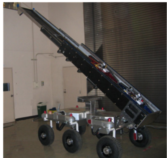
Fig.1 Slide ramp of large robot to lift-up small robots
