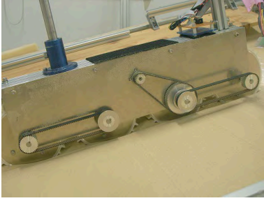
Figure 12: Slope test for inline four-wheel testbed
