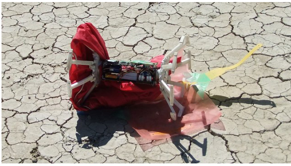
Fig. 10: WindMill-II was stacked into the parachute
