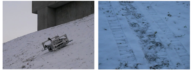
Fig. 4 Traverse on snow-covered slope
