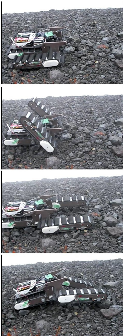
Fig. 5: Sub-track motion of Track Walker
