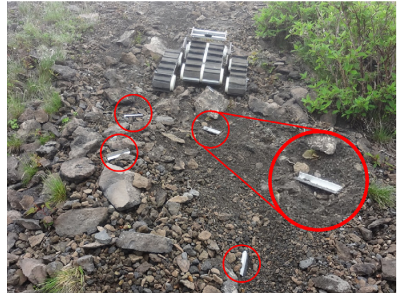
Fig. 4: Lugs come from TrackWalker-II
