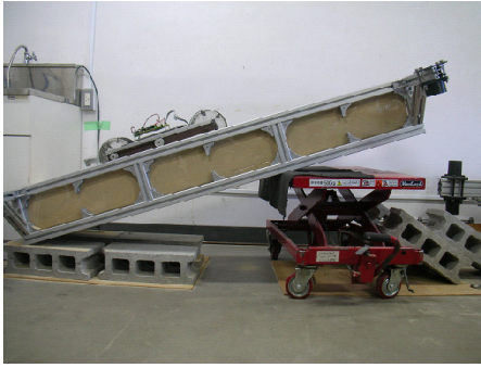
Fig. 8. Slope-climbing test; two-wheeled rover travels over a slope.
