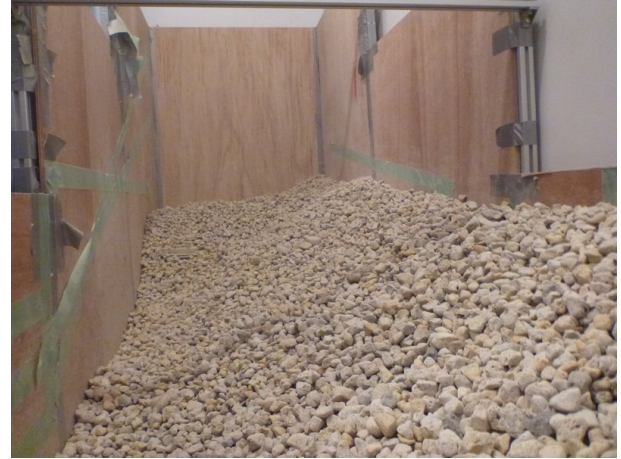
Fig. 8: Test field filled with pumice
