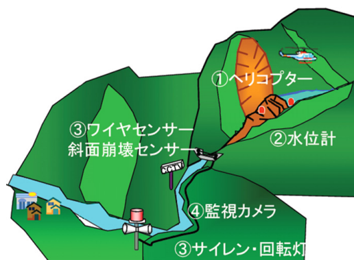
Fig. 2: Observation system of natural dam [3]
