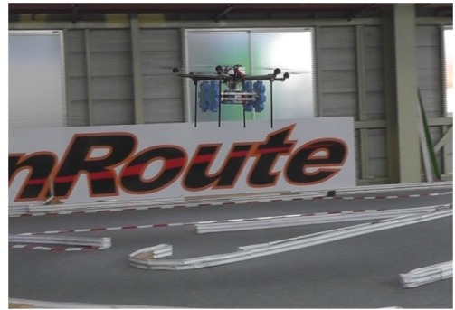
Fig. 10 An indoor flying experiment for multi-rotor UAV
