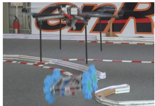
Fig. 11 Separation of "CLOVER" from the multi-rotor UAV
