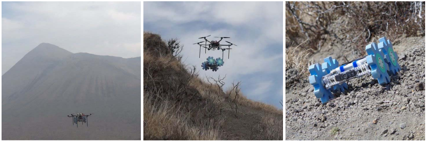
Fig. 10. Outdoor flying experiment in Shin-moe-dake (Mar. 11, 2013): In the left photo, the UAV (ZionPro 800) carries the ground robot (CLOVER). In the middle photo, the ground robot is released from the UAV. In the right photo, the ground robot traverses on the slope of the Naka-dake.
