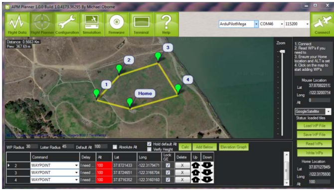
Fig. 5. Screenshot of GPS-based way point navigation based on ArduCopter software package. ( http://code.google.com/p/arducopter/ )
