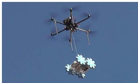
Fig. 1. Small mobile robot carried by a hexa-rotor UAV
