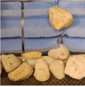
Fig. 3: Clogging of samples between roller and bucket
