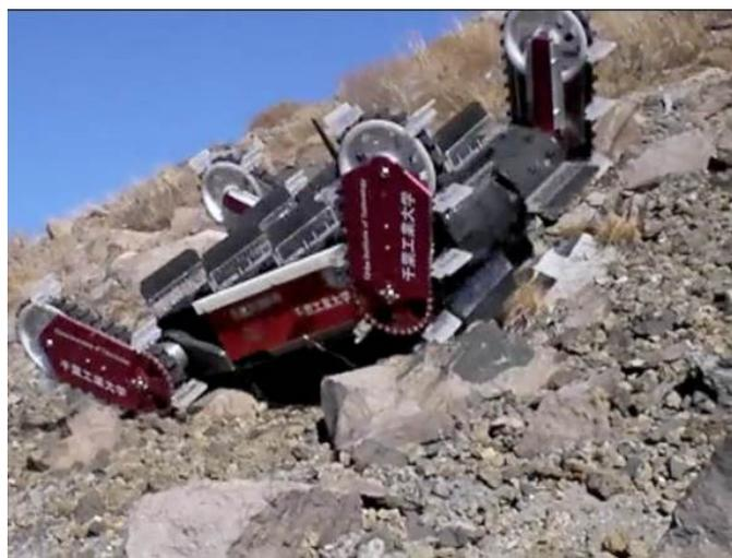
Fig. 1. Quince with flat lugs for volcano exploration: trying to traverse a weak slope on Mount Asama.
