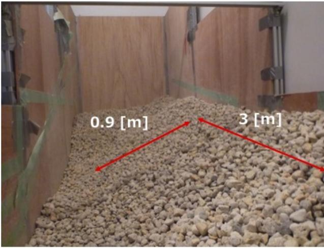
Fig. 9. Simulated volcanic field. The field was filled with pumice stones, and the slope angle was set manually.
