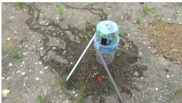
Fig. 6: Result of automatic permeability test on hard ground
