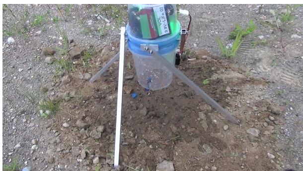
Fig. 7: Result of automatic permeability test on soft ground
