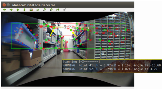
Fig.5 Suspended chain is detected.
