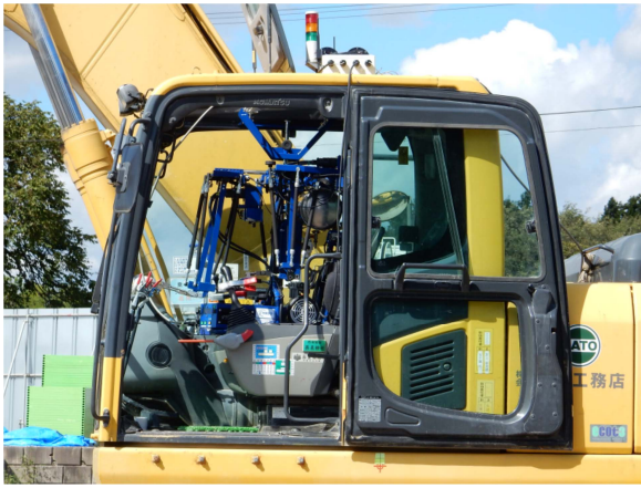
Fig. 2: SAM for Tele-operation of backhoe.
