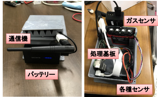
Fig. 3: An appearance of sensor body and inside of the apparatus.
